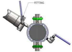
Fitting for priming "outlet side"
