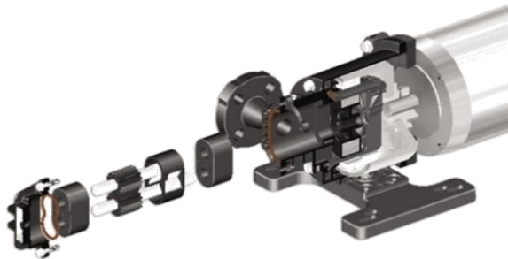
Figure 3 – The front pullout design of the Eclipse allows for the unit to be quickly repaired where it is installed without removing any attached piping
