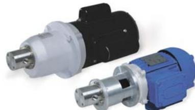
Material selection for Hydrogen Peroxide transfer pumps has been simplified due to its carbon incompatibility and product integrity issue. Decomposition into water and oxygen is accelerated by a wide variety of catalysts, especially in lower concentrations of Hydrogen Peroxide. Nickel, which is a major constituent of Hastelloy C, happens to be one of these catalysts. Therefore, Hastelloy C construction is generally not recommended for Hydrogen Peroxide applications because it will enhance this
