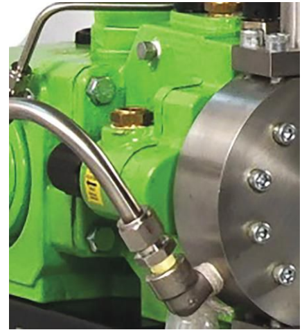
IMAGE 4: A nitrogen-ready design for a hydraulic diaphragm metering pump is a key consideration for TEAL applications.
